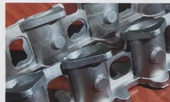
Manifolds pre and post fettling, where excess material is trimmed away and the surface cleaned.
