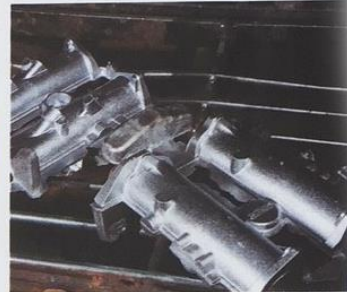
Throttle bodies as they appear out of the sand moulds.
