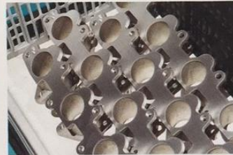
Completed manifolds ready for the stores.
