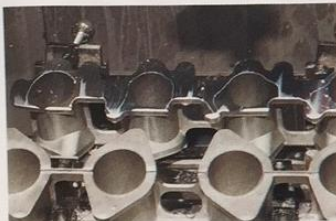
Rear manifold's mounting face machined, front to do.
