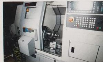
CNC controlled lathe used for boring throttle bodies to correct inner diameter.
