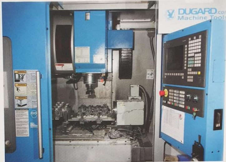
Four-axis CNC milling machine works on two manifolds at a time.
