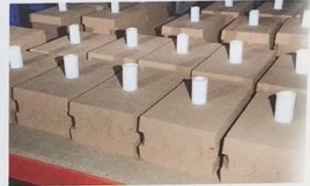
Two-piece moulds 'lock' together. White spout is where molten aluminium is poured in.
