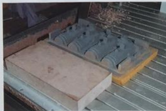
Wooden patterns are CNC milled using Rakutool composite modelling board.
