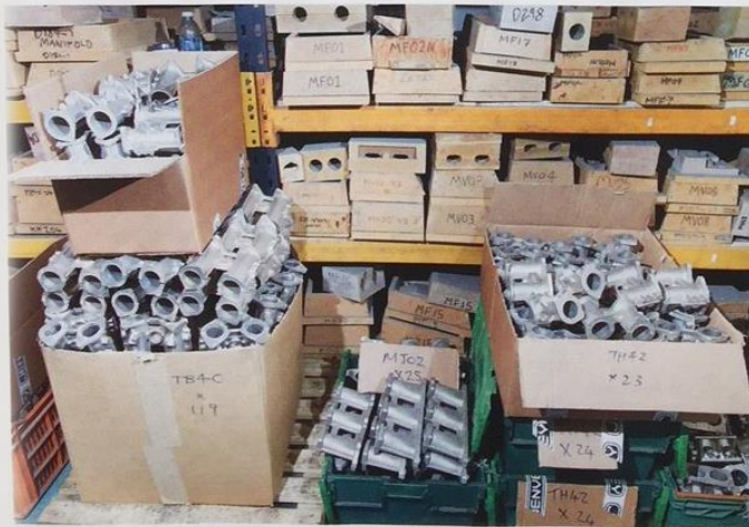
Throttle bodies and manifolds back from heat treatment. Patterns seen on the shelves behind.
