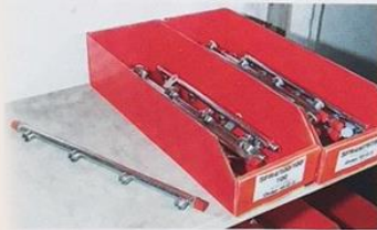
Fuel rails are sent away for plating.
