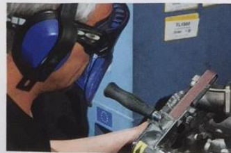
Fettling is done by hand, here with a belt sander.
