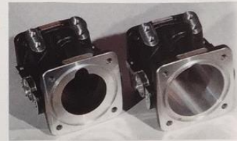
Left throttle body as created. Right example now bored out to customer specification.
