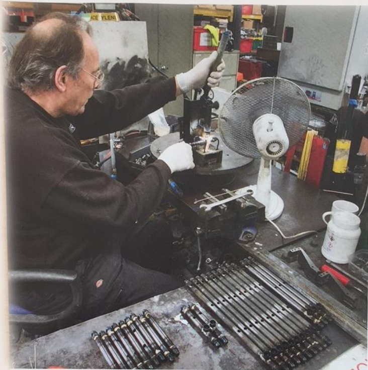
Pete in the process of creating steel fuel rails.
