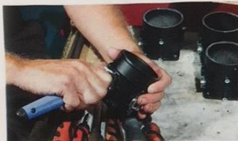
Despite the CNC machining, components are checked by eye and minor deburring may be needed.
