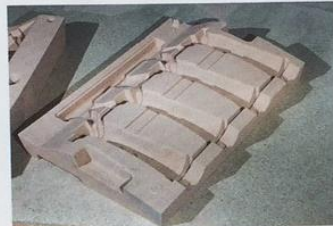
This is one half of the sand mould.
