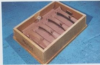
Outer lift-away frame is made from MDF. This is just one half of a product.
