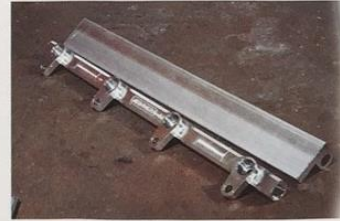
Same milling machine also creates billet fuel rails.
